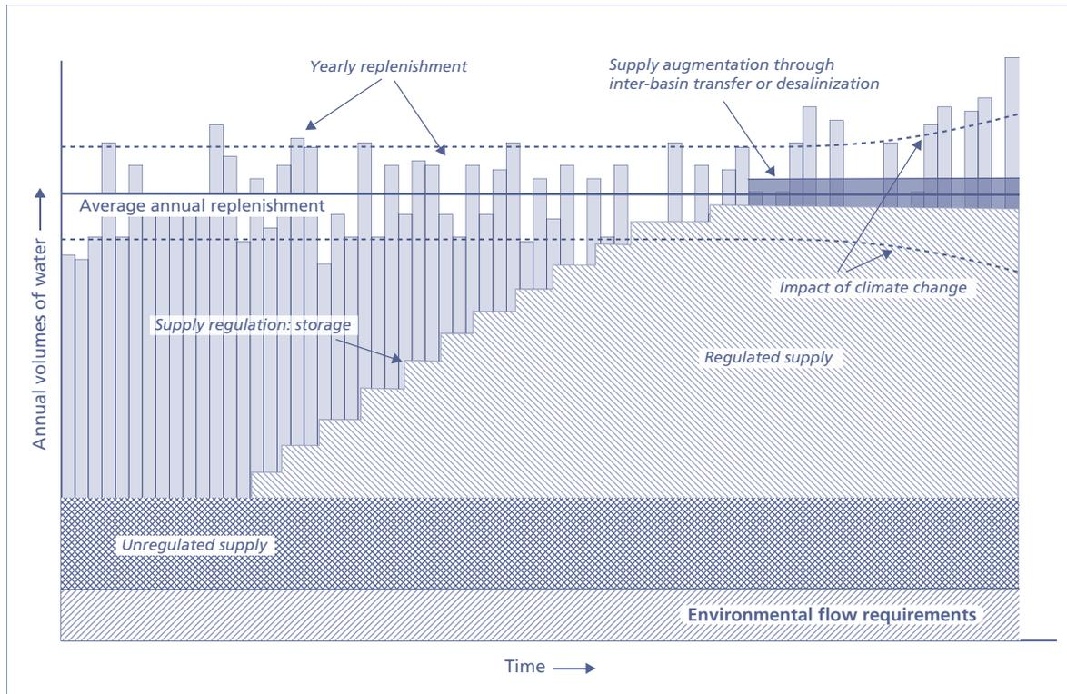
time and space, and inter-annual variability depend on climatic and geomorphological conditions. The geological conditions further determine the characteristics of groundwater recharge and storage. The availability of water is much less than the total water flowing in a system. It fluctuates from year to year, and only part of it is accessible for human use as a reliable source of constant supply.
